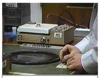
Cut or cleaved samples (~4 x 6 mm) are mounted face (good surface) down on a precision hand grinder's sample stub with LT- wax.
