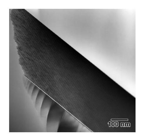
An x-ray mirror consisting of 45 layers of alternating Mo/amorphous Si (7.0 nm period) on a Si Substrate. The film was deposited using ion sputtering.
