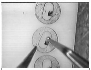
Place the folded grids on a Teflon block. Touch the end of the tweezers into the epoxy and place a small dollop of it on the vertical tab of folded grid.
