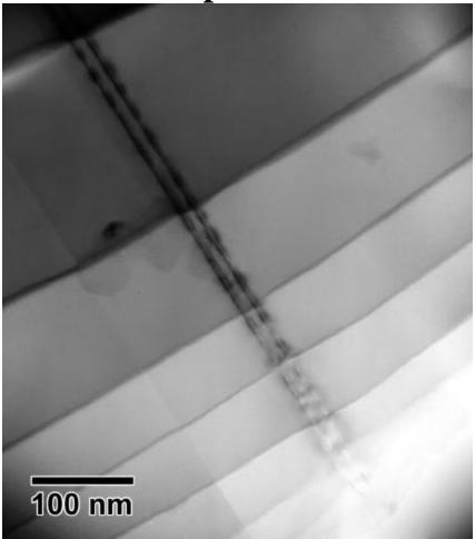
This figure shows a series of cleavage steps on a GaAs-based sample of InGaAs quantum dots. The steps range in length from approx. 70 to 200 nm. Quantum dot structures can be employed to enhance the performance of InGaAs based semiconductor lasers.
