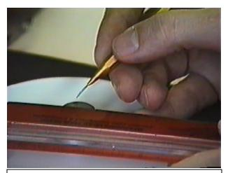
Along the scratch marks or with the aid of a protractor reticle, scribe lines with a straight edge. Multiple light passes are better than a single heavy one.
