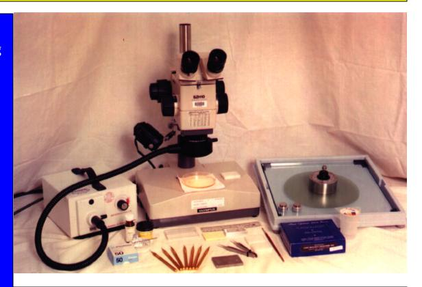
The total cost of the equipment and necessary supplies illustrated here to get started in using SACT is less than \$10k. In a typical TEM specimen preparation laboratory, most of these supplies are already available, making the initial investment in the technique minimal. Non-standard items include the mini-diamond scribes, the very sharp tweezers, the viscous epoxy, and the Teflon blocks.
