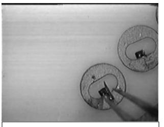
Pick up a cleaved sample and touch it to the epoxy on grid. Hold the grid down with a second pair of tweezers if needed.
