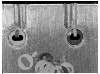
Style 1: Rotate the grid so that tweezers can get underneath the tabs and bend them up. Style 2: Flip them over and bend so that vertical tab goes thru hole.
