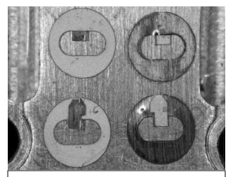
The two sides of the bending jig can make left- and right-handed grids in both styles. Style 1 is easier to make, but is not as tight and requires epoxy.
