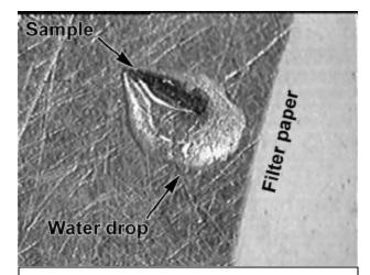
To remove the sample from water, hold tweezers vertically with points touching glass and gently tweeze sample. Place sample on Teflon block.
