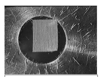
The thinned sample is approximately  $100~\mu m$  thick and has scratch marks running  $12\text{-}15^\circ$  to the cleavage directions.
