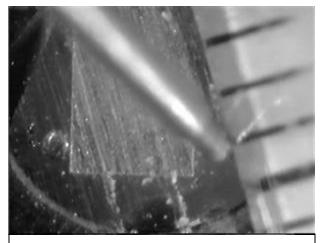
Scribe lines should be parallel and approximately 0.5 mm wide. Excess LT-wax around sample protects sample edges, diamond point, and mount.
