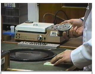
Insert stub into the grinder and set position of sample below the grinder's polishing surface.
