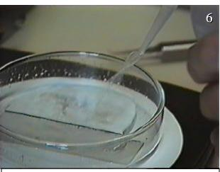
Permanently mount a glass slide in a Petri dish. Fill the dish with distilled water for each new sample. Thoroughly clean dish between uses.
