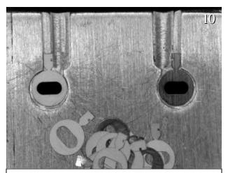
Grids are placed in the jig with the tabs on the ledge and held firmly against the wall with a pair of tweezers. The vertical tab part hangs over the ledge.
