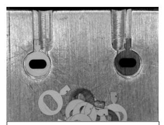
Bend the tabs down first. (This can be done first in the freestyle method, also.) Smooth the tab along the trough wall with tweezers to make a square bend.
