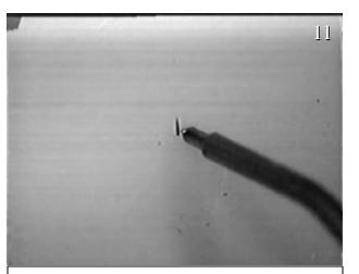
Very small pieces can be picked up with the diamond tip dabbed with epoxy.
