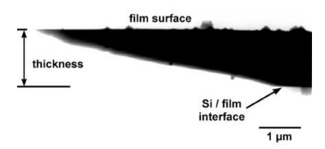
A pulsed laser deposited film of ZnO/WS<sub>2</sub>, a high temperature adaptive solid film lubricant. The sample has the "knife-like" SACT appearance, but is electron transparent along the edge. The film is amorphous and the striations are due to differences in the W concentration because of the small angular distribution of W in the ablation plume. This sample shows very clearly how the spherical particles, inherent to the PLD process, project their presence to the surface.
