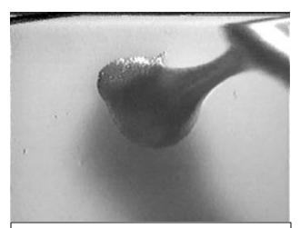
To test the epoxy for correct consistency, pull the rod up from the mix.
