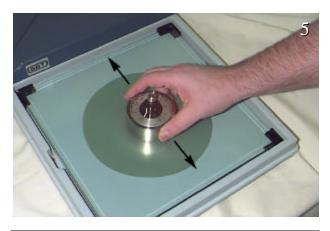
Alternative Method: The last grinding is done in a straight back and forth motion in the direction of the 12-15° estimated line on the sample.
