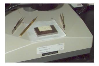
For the no-water approach, after fracturing along scribe lines (next step), place face up on the sticky part of a small Post-it<sup>TM</sup> note taped to a block.
