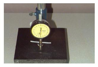
When  ${\sim}50~\mu m$  away from the desired thickness, stop. Measure thickness with a "zeroed" grinder or independently with calipers or dial indicator (shown).
