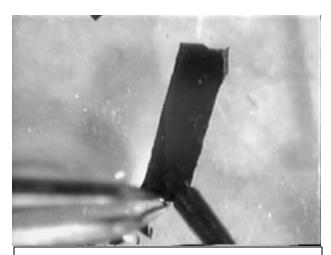
By gently applying pressure, a cleavage line will propagate up and intersect the edge at a 12-15° angle.
