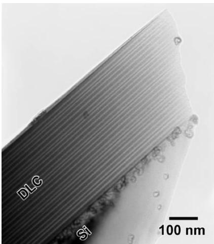
This figure shows a pulsed laser deposited diamondlike carbon film on a silicon substrate. The film is amorphous. The striations are density variations in the film and are caused by angular variations in the ablation plume as the laser is rastered over the target.
