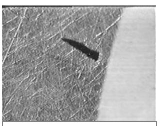
Touch the drop of water with the edge of the filter paper. The water will wick away from the sample and the Teflon block.
