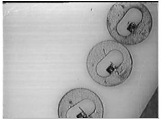
Finished samples all in a row! Cure the samples on the Teflon block with the temperature of the hotplate around 100-125°C and pop them into the TEM.
