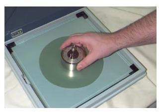
An alternative to the polishing wheel is the use of a flat, glass plate arrangement using diamond film abrasives.
