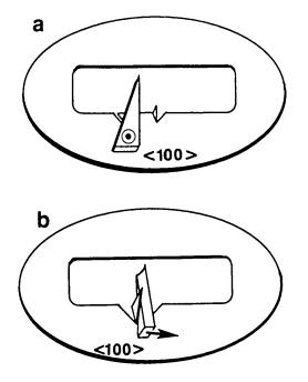
If the sample is epoxied to the vertical tab very carefully, then the tab itself can be bent over. This allows the examination of the sample in both a plan view (a) to measure thickness of the steps and XTEM view (b). The sample can also be examined in a high resolution SEM very easily in this manner.
