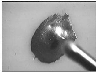
If the height of epoxy is about 1 cm when it breaks, then the consistency is just right. If not, add a little of what is needed or start over.
