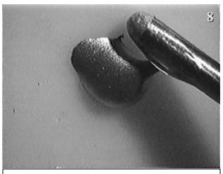
To mix the H-22 silver epoxy in the quantity needed, put a small drop of silver-filled resin onto Teflon. Touch a 1/16" rod to hardener and add to drop.
