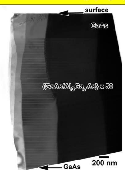
A Multiple Quantum Well structure grown by Molecular Beam Epitaxy showing the thickness terraces. The GaAs buffer, 50 periods, and GaAs cap are all seen with very small variations in thickness within a step.
