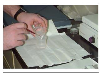
Remove the samples by heating or soaking in acetone. Use a brush to remove the delicate samples. A 2nd rinse in fresh acetone is recommended.
