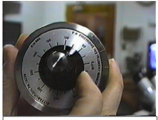
Set grinder to final thickness. Mentally note which mark is parallel to sample direction and estimate a line 12-15° from it. Here, each division is 18°.
